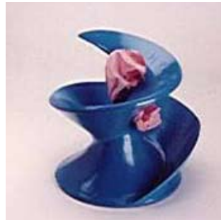
Velocity of incoming flow sweeps rags and fibre along blade towards centre of impeller
