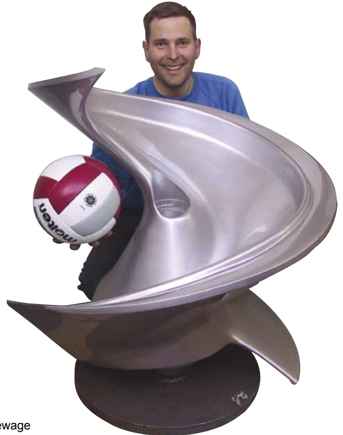
Impeller from 700 mm discharge raw sewage pump
