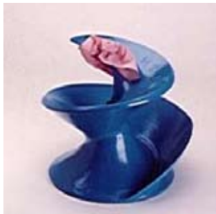
Rags and fibre initially contact leading edge of blade
