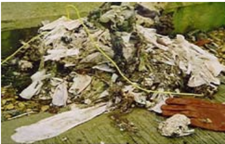
Typical material removed from a 300mm conventional sewage pump
