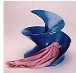
At centre of impeller the material makes a smooth transition from the blade to being deposited into the impeller channel thereby passing freely through the pump
